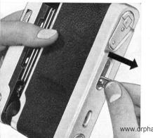
like unloading and changing partly exposed films (see pages 22 and 23) is specially easy and quick, for the camera back is separate from the body. You can therefore remove it completely and carry out all the necessary operations without obstruction.
