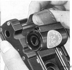
The VITESSA takes standard daylight cartridges of perforated 35 mm. film. Although these cartridges are light-tight, it is best not to handle them in too strong light. Therefore load and unload the camera in the shade — even the shadow of your own body will do.
