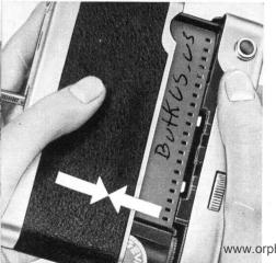
Push the camera back and body together again (see illustration). Keep them pressed together while you turn back the latch and fold it down.
